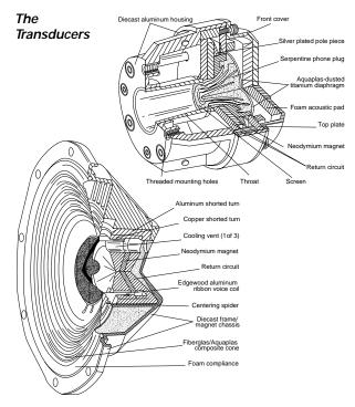
Figure 2. Cutaway view of JBL 475Nd high-frequency compression driver. Note the curved (equalized) paths from the diaphragm to the driver's output.
